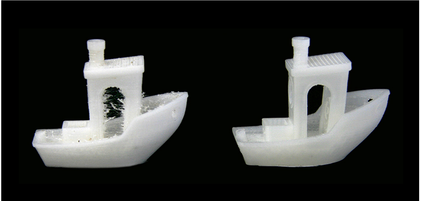
3D Benchy printed with undried and dried filament, using same printing settings and same g-code
